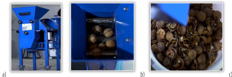
Figure 7. GRK 300 nutcracker a) General view, b) Power supply system, c) Overview broken walnuts ( https://tmagro.com.ua/ )
