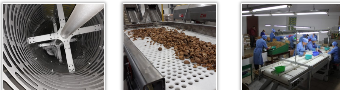
Figure 10. Constructive solutions for calibrating nuts and walnut kernels, a) with cylindrical sieve, with flat sieve, c) sorting table
