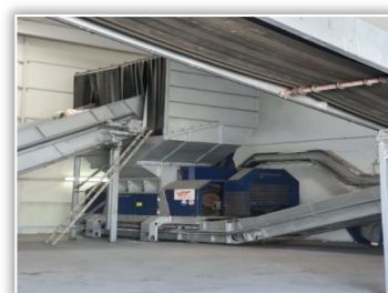
Figure 4 – Mixing shredding plant in two successive stages – the shredder
