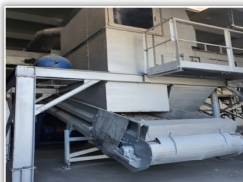
Figure 4 – Mixing shredding plant in two successive stages – the shredder
