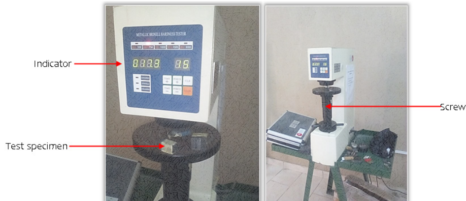
Figure 1: Brinell hardness test of test material
