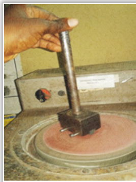
Figure 6: Test specimen under wear test
