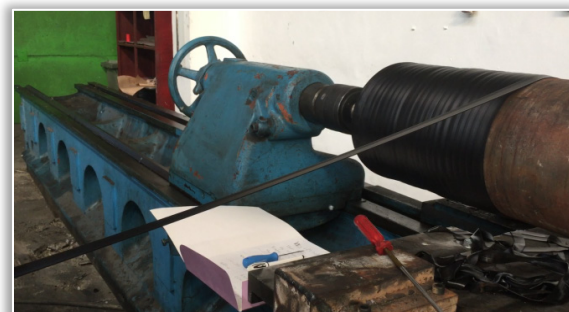
Figure 2. The metallic drum on which the thin rubber band is wrapped – manual winding stage
