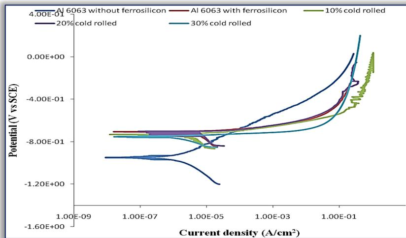
Figure 6: Potentiodynamic polarization curve of cold rolled aluminium alloys in 3.5wt % NaCl solution
