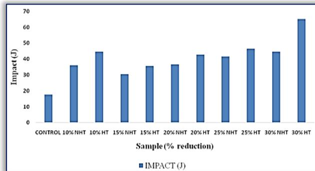
Figure 3. Impact Stress of Heat treated and non-heat treated cold rolled samples
