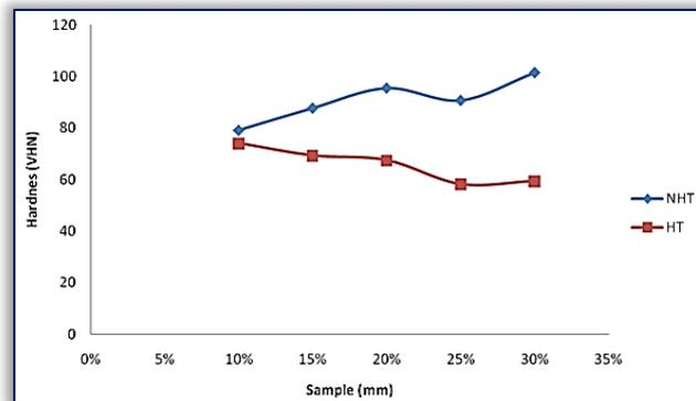
Figure 4: Comparison of heat-treated and non-heat-treated cold rolled Samples
