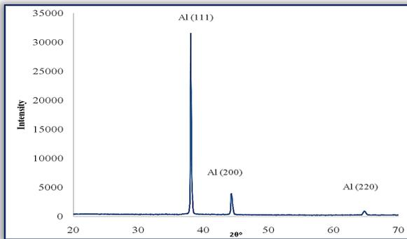
Figure 1. XRD pattern of as received Al 6063
