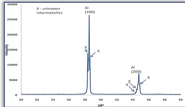
Figure 2. XRD pattern of Al 6063 alloyed with ferrosilicon
