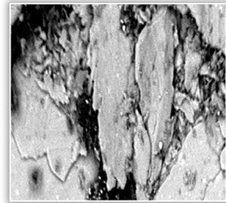
Plate 3: 20 % cold rolled sample
