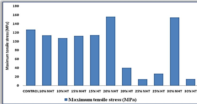
Figure 5: Maximum Tensile Stress of Cold Rolled and Heat-treated samples
