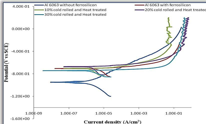
Figure 7: Potentiodynamic polarization curve of cold rolled and heat treated aluminium alloys with various degrees of cold rolling
