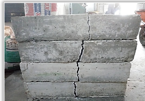
Figure 9. Failure mode of the unreinforced concrete beams containing metakaolin
