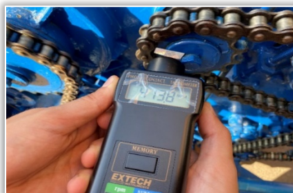
Figure 6. Aspects during the measurement of the revolutions of the working organs of the vine shoots baling machine: a) with contact; b) without contact
