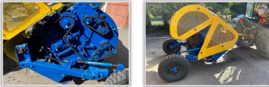
Figure 5. Aspects during checking the operation of the bale unloading system
