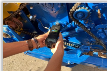
Figure 6. Aspects during the measurement of the revolutions of the working organs of the vine shoots baling machine: a) with contact; b) without contact
