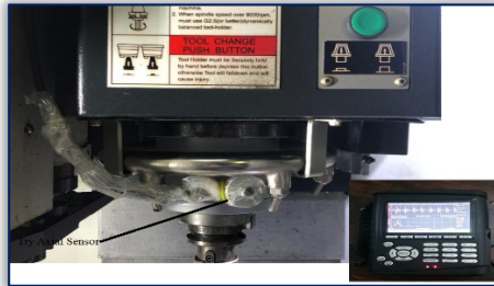
Figure 1.(a) CVM milling Machine with CoCo80 Dynamic Signal analyzer with Try Axial Sensor
