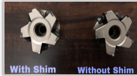
Figure 1.(b) Face milling tool 63 mm dia with shim and Without shim face mill
