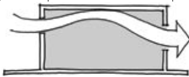
Figure 3c. Inlet placed high directs flow upward resulting in loss of cooling effect
