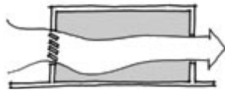
Figure 3b. Louvers placed in a downward position at the inlet diffuse airflow
