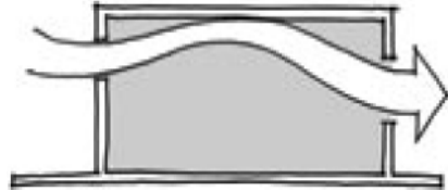
Figure 3c. Inlet placed high directs flow upward resulting in loss of cooling effect.
