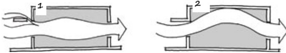
Figure 3e. 1. Providing a slot between a canopy or 'eye-brow' can increase downward pressure and result in a more comfortable air flow within a room. 2. Solid overhangs, or 'eye-brows', directly over a window can direct airflow upward away from the occupied zone of a room.
