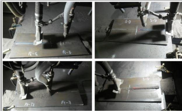
Figure 4. Submerged arc welding process of specimens
