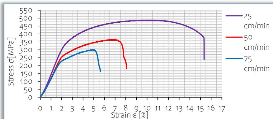
Figure 7. Stress–strain curves
