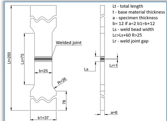
Figure 5. Tensile test specimen characteristics [12]
