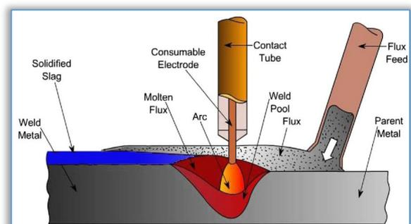
Figure 1. The principle of submerged arc welding [6]
