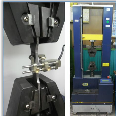
Figure 6. Strain test equipment
