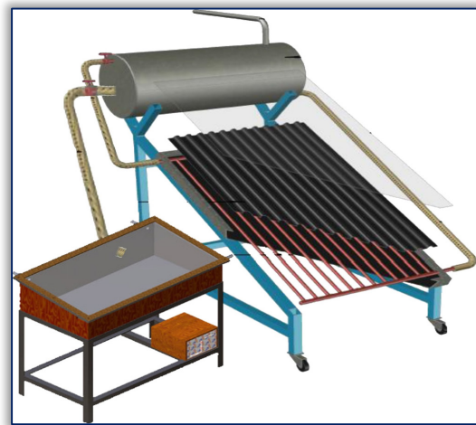
Figure 1: sketch of a combined solar water heater and water distiller
