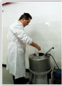
Figure 6 – Sludge centrifugation, on a laboratory centrifuge
