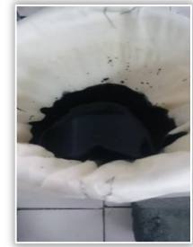
Figure 5 – Filtration on a bag filter to obtain sludge
