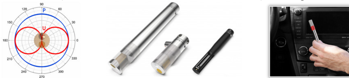
Figure 6. Combined sensor for noise visualization [17]
