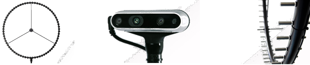
Figure 2. Microphone arrays of noise visualization tools – Ring72 AC Pro [11]
