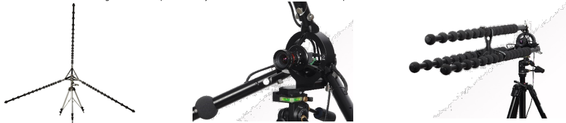
Figure 4. Microphone arrays of noise visualization tools – Star48 AC Pro [11]
