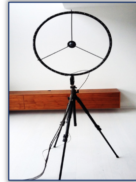
Figure 7. Installed acoustic camera during measurement
