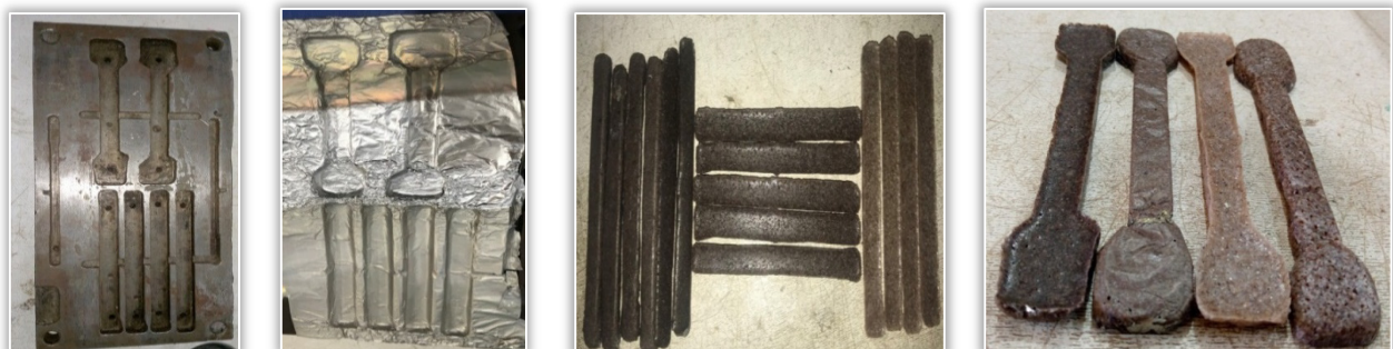
Figure 1. Nanocomposites production (a) mold (b) aluminum foil-lined mold (c, d) produced nanocomposite samples
