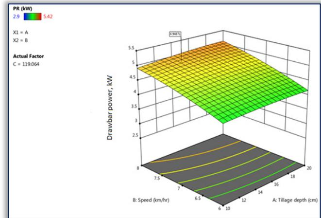
Figure 1. Response surface plot of working width, cutting depth and operational speed against power requirement of the disc plough in sandy–clay soil
