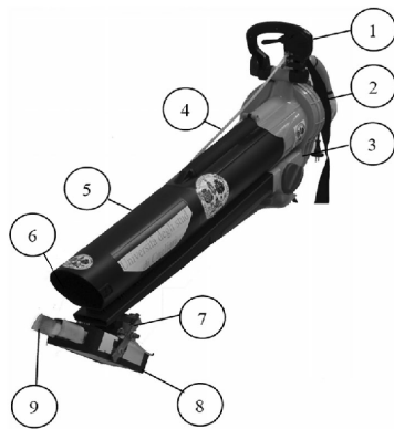
Figure 5 – Portable automatic system for harvesting saffron flowers (Manuello Bertetto A. et al. 2014)
