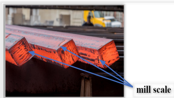
Figure 6. Formation of waste known as mill scale on the surface of continuously cast ingots [23]
