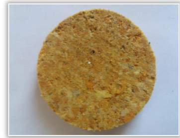
Figure 13. Material Ekomolitan after pressing
