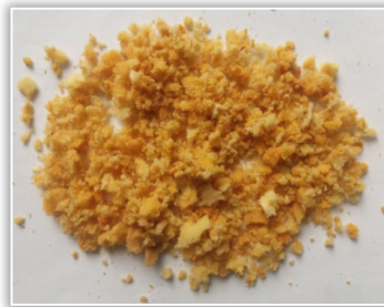
Figure 12. Ground fraction of PUR foam
