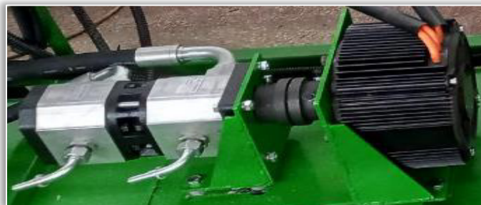
Figure 6 – The inverter and the electric motor mounted on the harvester during indoor tests
