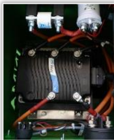
Figure 6 – The inverter and the electric motor mounted on the harvester during indoor tests
