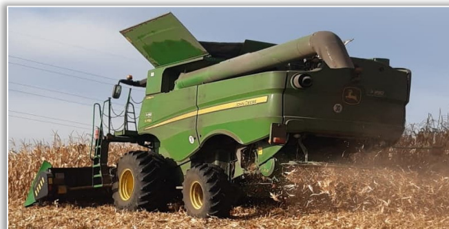
Figure 5 – Maize harvesting maize with chopping and spreading on the ground of vegetable residues
