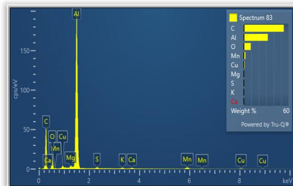
Figure 6. EDS profile for the sample at spectrum 82 and spectrum 83.
