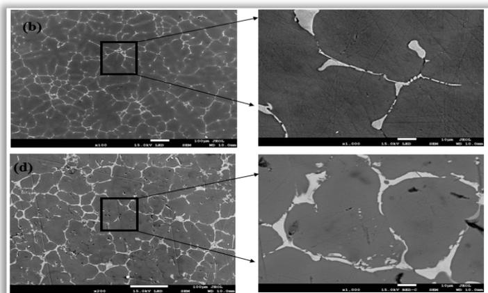
Figure 3. SEM photomicrograph of (b) Al–90%/Cu–7.5%/Al<sub>2</sub>O<sub>3</sub>–2.5% and (d) Al–90%/Cu–2.5%/Al<sub>2</sub>O<sub>3</sub>–7.5% sample composites
