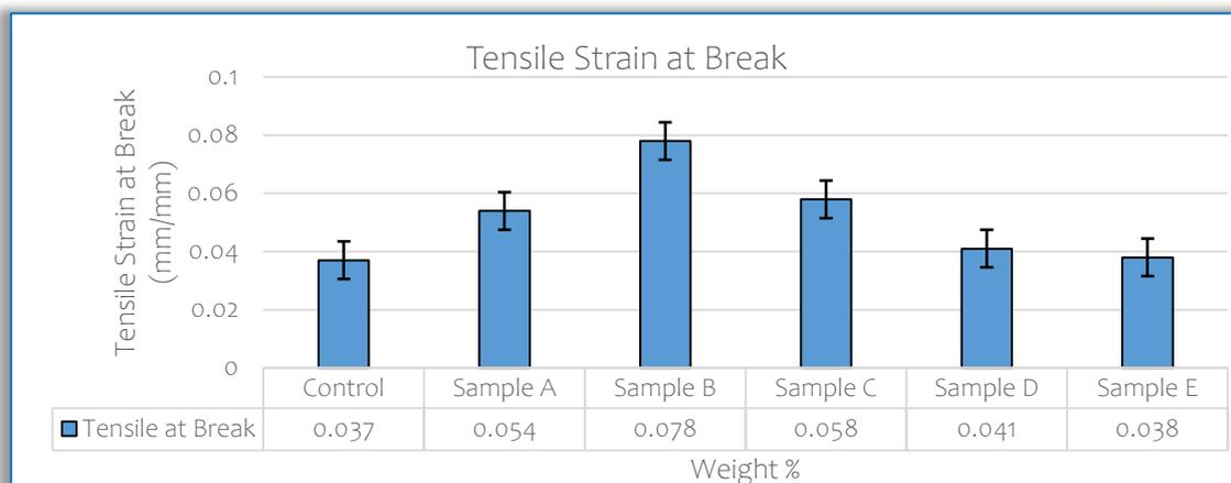
Figure 9. Variation of tensile strain at break with percentage weight of each sample
