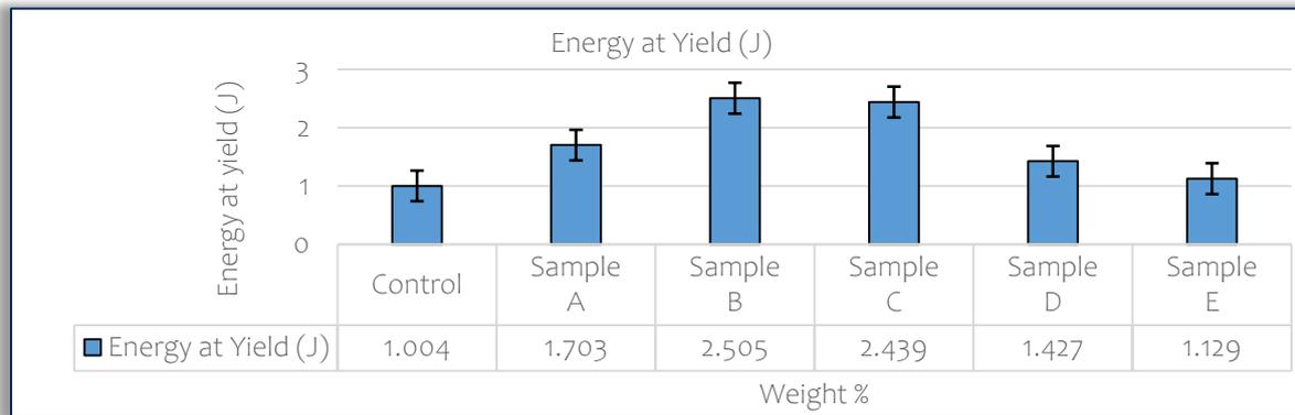
Figure 12. Variation of energy at yield with percentage weight of each sample.
