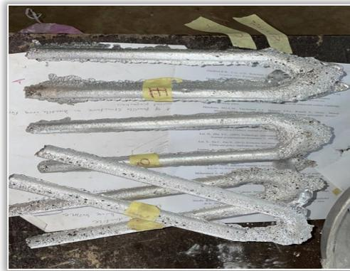
Figure 1. As-cast aluminum based composites.
