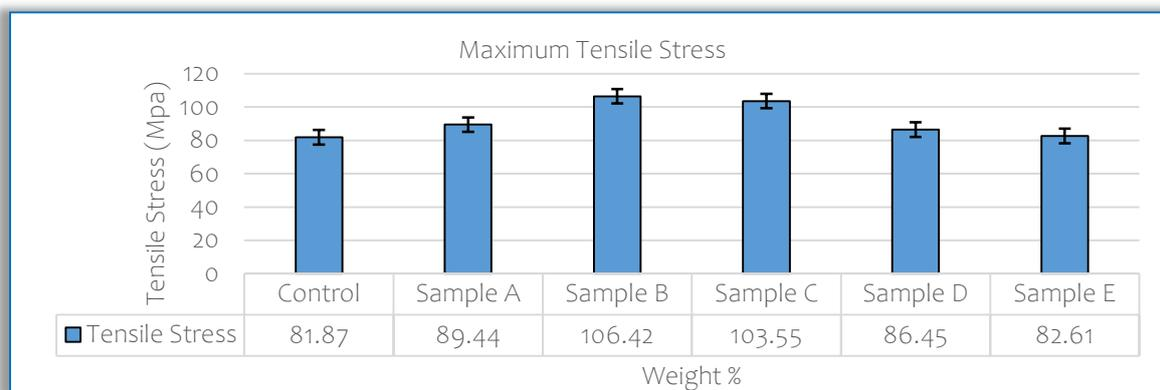
Figure 10. Variation of maximum tensile stress with percentage weight of each sample
