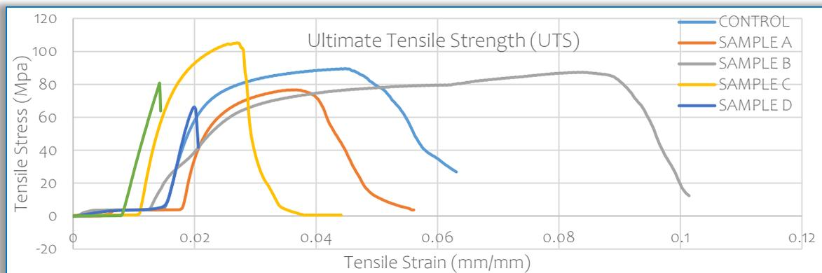
Figure 8. Variation of tensile stress with tensile strain of composite samples
