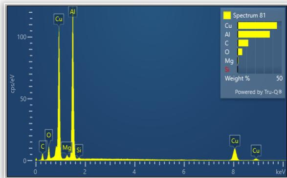
Figure 5. EDS profile for the sample at spectrum 81
