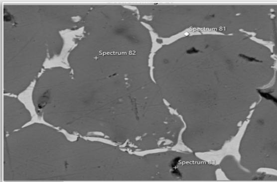
Figure 4. Secondary electron image of Al-90wt% matrix with Cu particles of 2.5wt. % and Al<sub>2</sub>O<sub>3</sub> reinforcement of 7.5wt% showing different spectra
