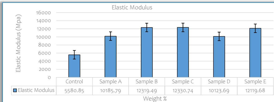
Figure 11. Variation of elastic modulus with percentage weight of each sample.
