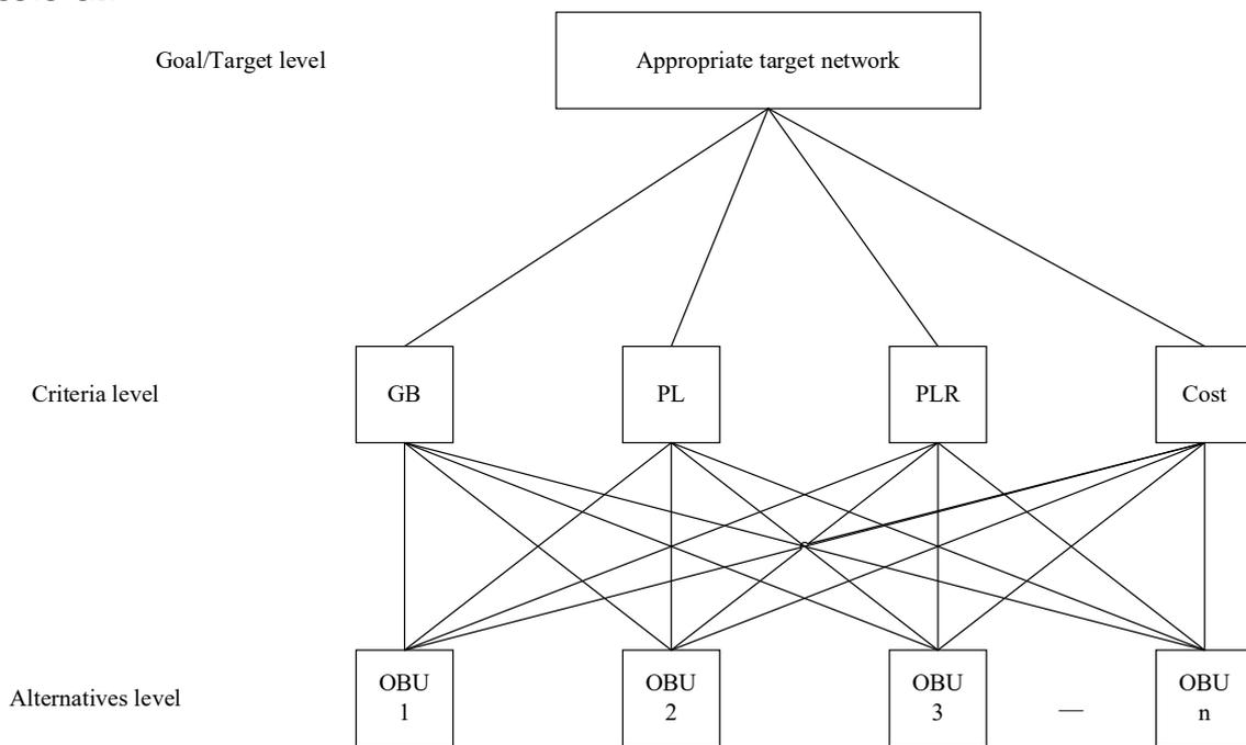
Figure. 1: Hierarchical Structure for V2I Handover Decision
