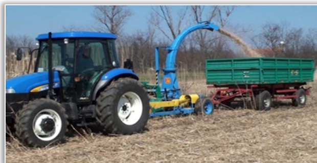
Figure 7. Tractor unit – towed combine for harvesting [22] MISCANTHUS stalks, during work
