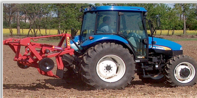
Figure 5. Technical equipment for harvesting Miscanthus rhizomes ERR [13]
