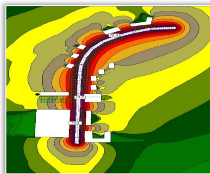
Figure 7. 3D Watson street model with noise levels in dB
