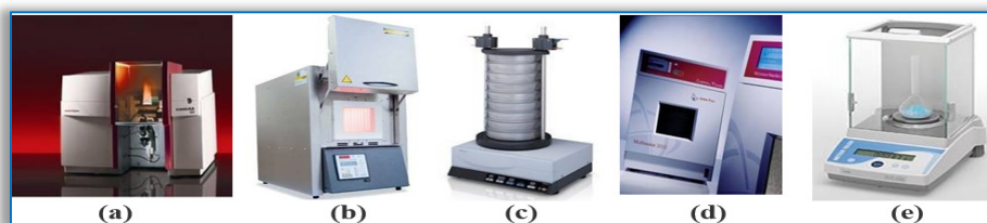
Figure 4. Laboratory equipment for testing raw materials and finished products: (a) High resolution spectrometer; (b) High temperature compact oven; (c) AS 200 Control sieve analyzer; (d) Microwave system for mineralization under pressure; (e) Analytical balance type AL204, Mettler–Toledo [11,12,18]
