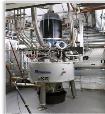
Figure 3. A 1-MW, 150-GHz gyrotron used to heat plasma in the Wendelstein 7-X stellarator fusion experiment in Germany [15, 16] (CC BY-SA 4.0).
