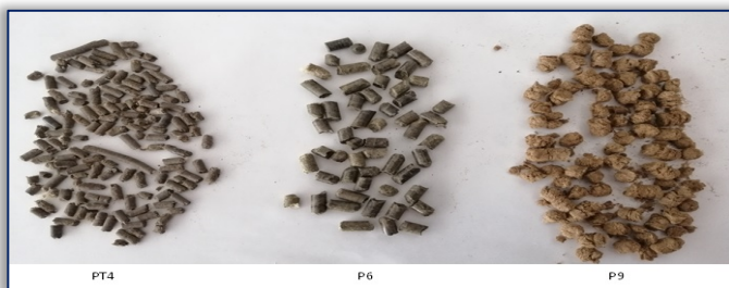
Figure 2 – Wool pellets used in experiments: PT4–imported pellets with 4mm diameter; P6–raw wool pellets with 6 mm diameter; P9– clean wool pellets with 9 mm diameter
