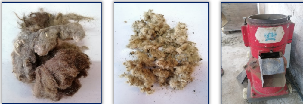
Figure 1 – Wool and press used for pellets: a) raw wool, b) grounded wool, c) pelleting press
