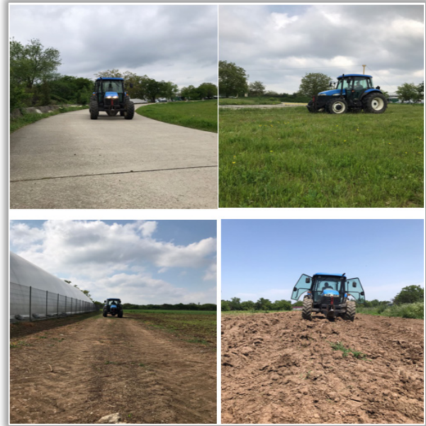
Figure 1 – Performing experimental tests on terrain types according to the experimental protocol, at speeds of 6 and 12 km/h: a) straight terrain; b) uncultivated land; c) uneven ground; d) plowed land
