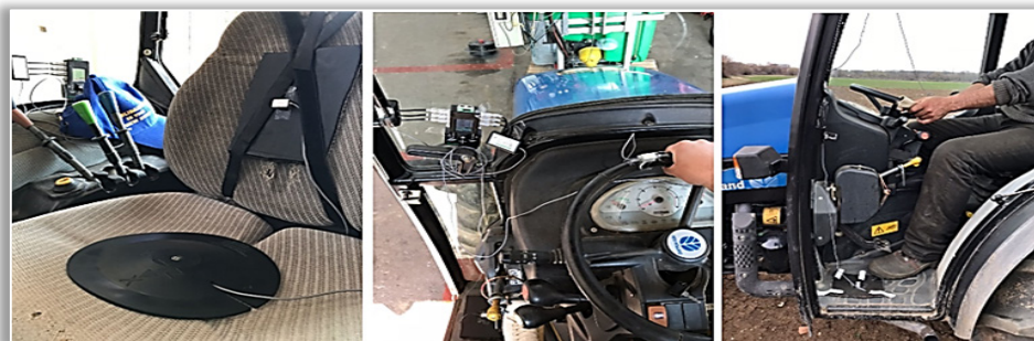
Figure 2 – Installing triaxial accelerometers on the surface of the tractor's seat, on the seat-back and on the cab floor at the support leg
