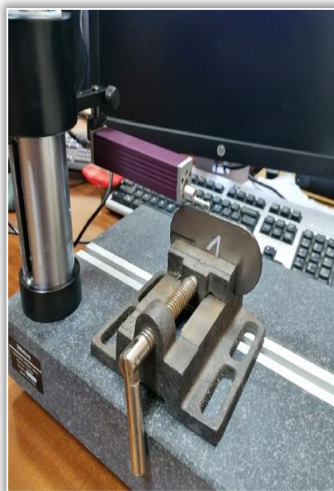
Figure 4. Presentation of the measurement of surface roughness on samples using the Mitutoyo SurfTest SJ-210 instrument
