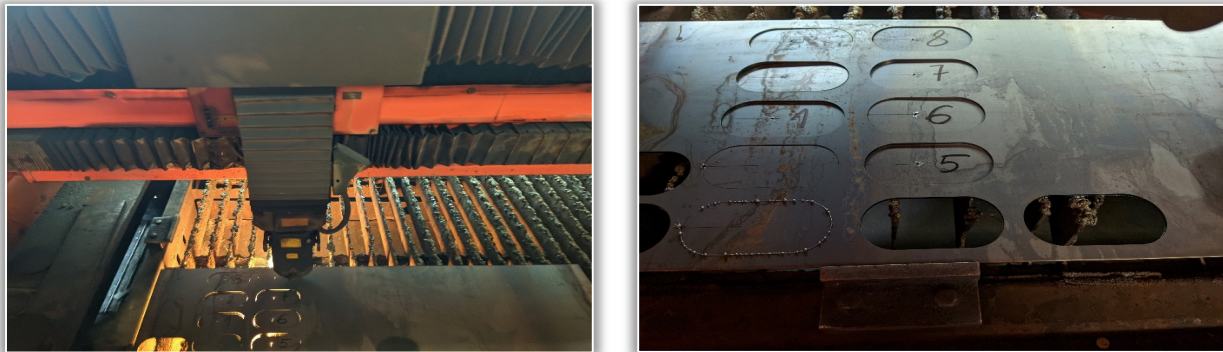
Figure 3. Illustration of the laser cutting process and the appearance of the sample after cutting from the sheet metal
