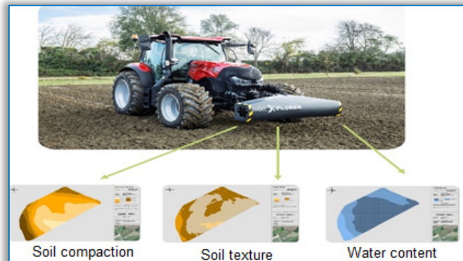
Figure 4 – Scanning of the soil, regarding its degree of compaction, texture and humidity
