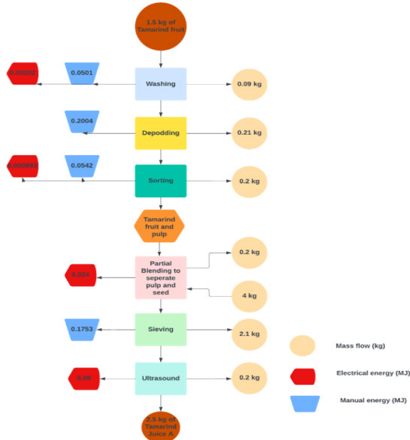
Figure 1: Mass and energy balance for production of tamarind juice drink ultrasound treated without seed (UPST)
