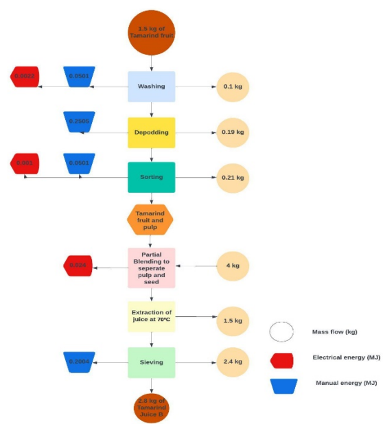
Figure 2: Mass and energy balance for production of tamarind juice drink pasteurized treated without seed (HEST)
