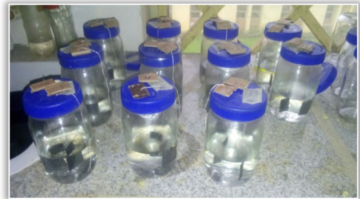
Figure 4: Immersion of specimen in hydrochloric acid
