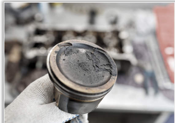
Figure 2. Deposits on engine components [12]
