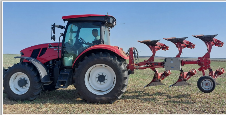
Figure 1 – Prototype of an innovative vibrating system for plows with bodies in operation and in production
