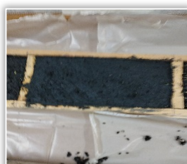
Figure 2 – bricks made with corn cobs – recipe 2
