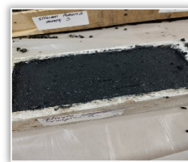
Figure 4 – bricks made with sunflower residues – recipe 2
