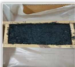
Figure 1 – bricks made with corn cobs – recipe 1
