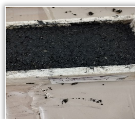
Figure 3 – bricks made with sunflower residues – recipe 1
