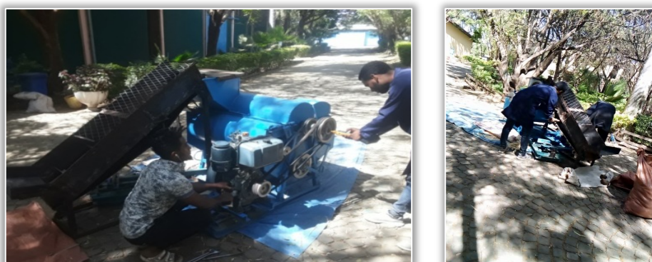
Figure 6. Picture of during the incorporation of drum speed with conveyor speed adjustment
