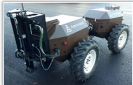
Figure 12 – Articulated platform prototype with soil sampling mechanism (Leemet, T., et al, 2018)
