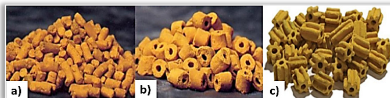
Figure 2. Shapes of the vanadium pentoxide catalyst. a) Pellets, b) Rings, c) Stars [8]
