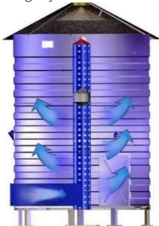
Figure 2 – Central column ventilation
