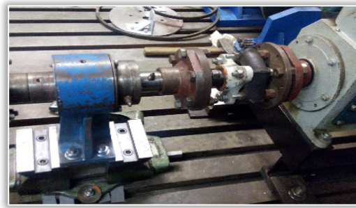
Figure 10. Mounted Hardy flexible shaft coupling in the test mechanical system
