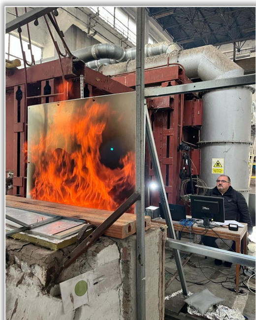
Figure 1. Experiment "0.5mm metallic protection sheet exposed to the action of temperature"
