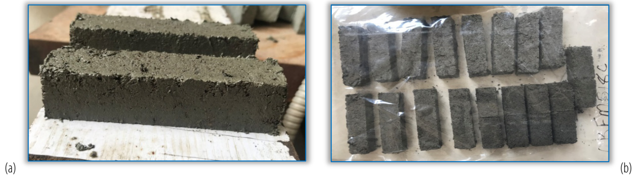
Figure 2: (a) Composite brick produced and (b) Curing of composite bricks in polyethylene bags
