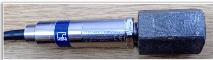
Figure 4. Pressure sensor and transmitter HBM 1-P3IC/3000 bar with adapter.
