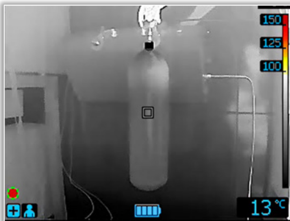
Figure 12. Thermovision image – measuring the temperature of the steel bottle on the console of the „air bank” (at the beginning of filling) [4].
