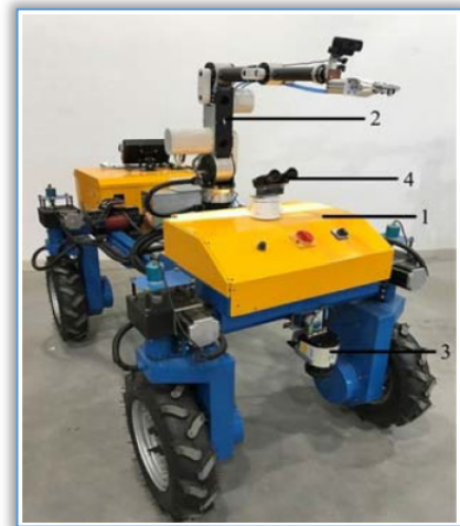
Figure 5 - Robot for tomatoes harvesting (Wang et al., 2017): 1 - mobile platform; 2 - harvesting system; 3 - navigation; 4 - artificial vision system
