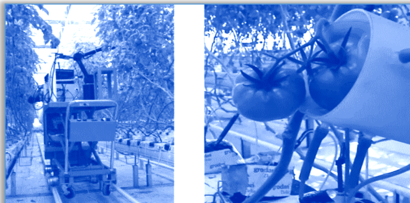
Figure 4 - Robot for tomatoes harvesting through suction (Wang et al. , 2022)
