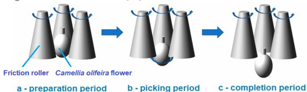
Figure 9 – The phases of the harvesting process simulated using the considered model. [adapted after 27]
