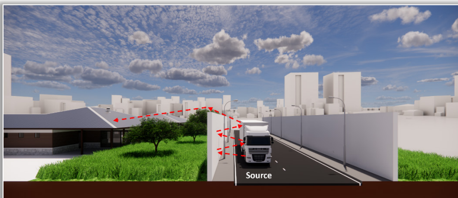
Figure 8. Multiple reflections between the noise barrier and the truck
