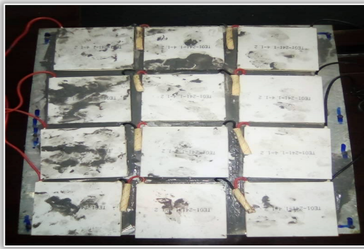
Figure 4. Modules attached to receiver plate
