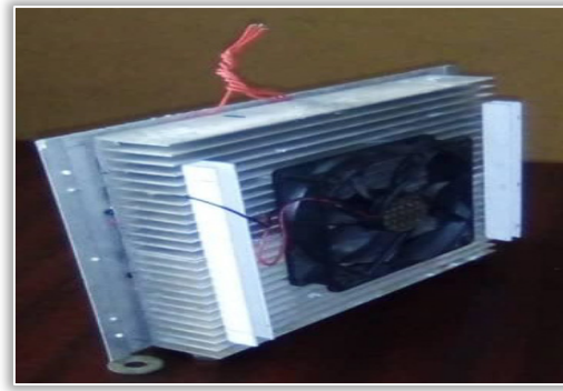
Figure 5. Assembly of Receiver plate, modules heat sink and cooling fan
