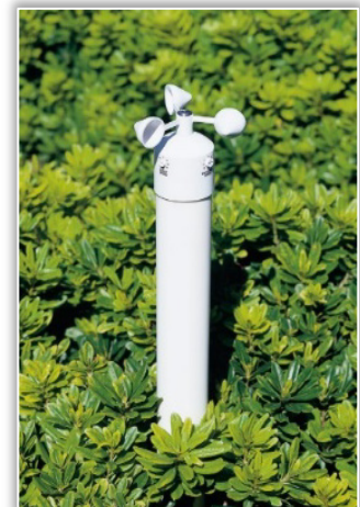
Figure 6: Wind sensor (made by Hunter Industries) for use in the landscape Source: Gotcher et al. (2017)
