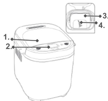
Figure 1 – Tefal Pain Plaisir PF220 bread maker: 1 – cover; 2 – control panel; 3 – kneading bowl; 4 – kneading arm (Munteanu et al., 2019)
