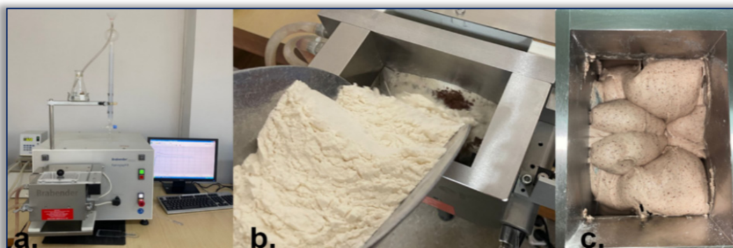
Figure 2 – Brabender Farinograph and dough mixing process during rheological tests
